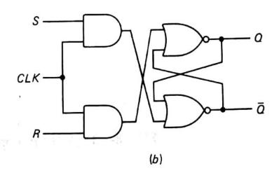
FIG. 8-11 Two different realizations for a clocked RS flip-flop
