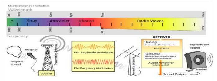
In FM radio stations transmit broadcast information by changing the frequency of the carrier wave. The strength of FM waves is always the same and is in megahertz. Mega=million
