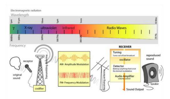
In AM amplitude changes but frequency does not. AM frequencies range from 540,000 Hz to 1,6000,000 Hz usually listed in kHz.
