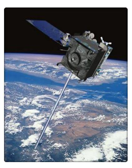
Thousands of satellites orbit Earth. A radio or TV station sends microwave signals to the satellite which amplifies the signal and sends it back to a different place on Earth. Satellite uses dif freq to send & receive.
